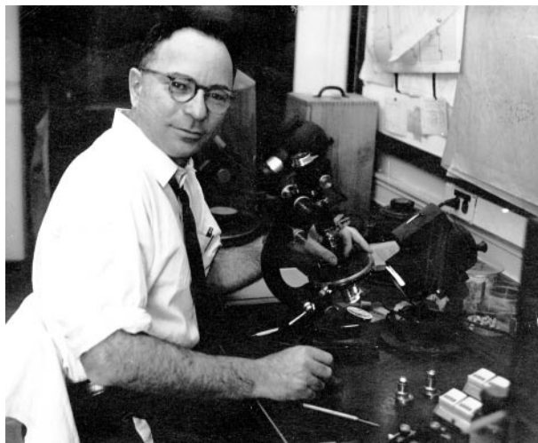
Figure 3. Felix Chayes at the petrological microscope (?1951). Note counters used for recording modal analysis counts in lower right. Reproduced with permission of the Geophysical Laboratory, Carnegie Institution of Washington.
