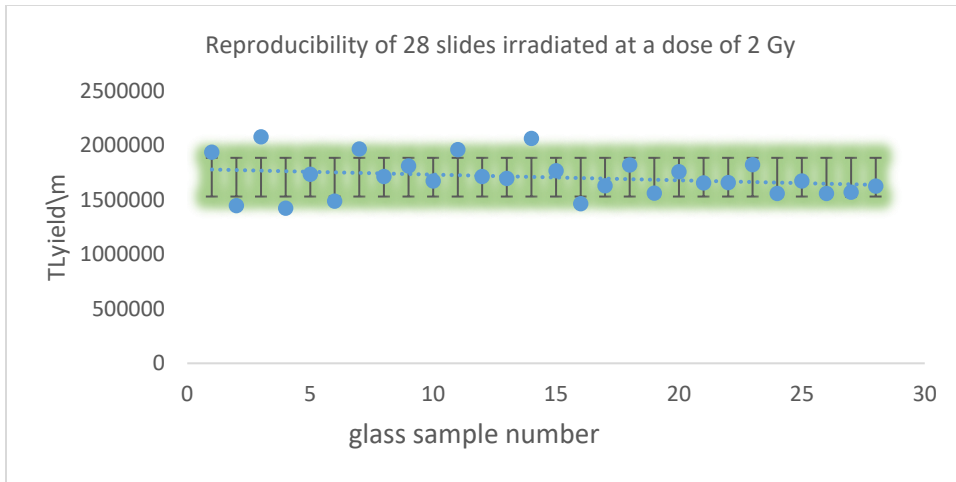
Figure 8. Reproducibility of the second group of glass slide samples (28 in all); outliers are easily screened out in such an exercise.
