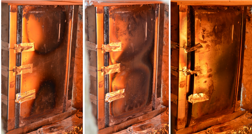
Fig. 17. Typical deformation of the steel sheet on the heated side: (a) during the initial period of heating; (b) during the later stage of heating; and (c) in cases of spalling of in-filled concrete.
