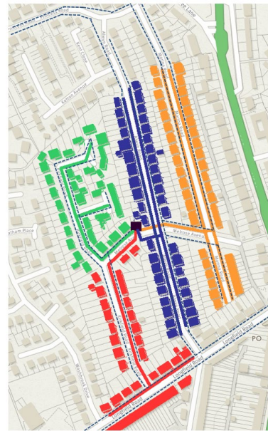
Figure 4 – Low-density network layout, showing 292 properties including semi-detached, detached and terraced housing. The secondary 500 kVA transformer is in the centre and supplies four colour coded electricity feeders/properties. Dashed lines indicate low pressure gas pipework.
