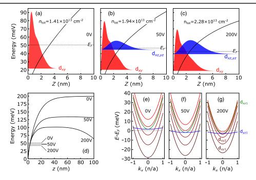
FIG. 3. (a)–(c) S-P calculations confining potential profile (solid line), Fermi energy (dotted line), and spatial distribution of mobile electrons occupying  $d_{xy}$  (red) and  $d_{xz,yz}$  (blue) bands at (a) 0, (b) 50, and (c) 200 V. (d) Confining potential and Fermi energy in a larger range. (e), (f) S-P calculated subband dispersions in parabolic approximation at (e) 0, (f) 50, and (g) 200 V.
