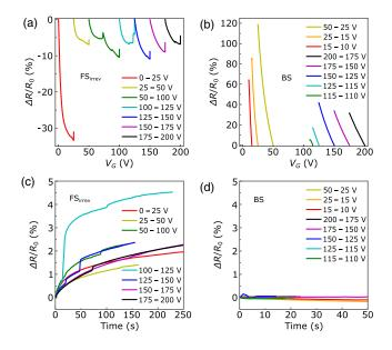
FIG. 5. (a), (b) Dynamic change of  $R_s$  during  $V_G$  sweeps in (a) FS<sub>irrev</sub> and (b) BS regimes.  $V_G$  was swept at a rate of 0.1 V/s.  $R_s$  measurements kept on going for several minutes after the stabilization of  $V_G$ . (c), (d) Dynamic change of  $R_s$  after  $V_G$  sweeps in (c) FS<sub>irrev</sub> and (d) BS regimes.
