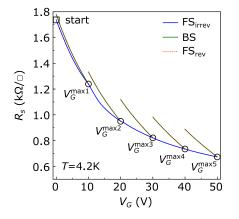
FIG. 4.  $V_G$  dependence of  $R_s$  at 4.2 K. The sweep order is similar to that in Fig. 1(a). Backward sweeps were performed from 10 to 50 V. Note that BS and FS<sub>rev</sub> overlap perfectly.
