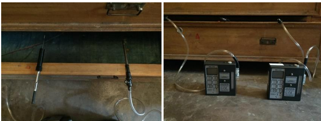
Figure 12-1. Sampling of mould VOCs in a historic church using carbon-sorbent tubes connected to an electronic pump.
