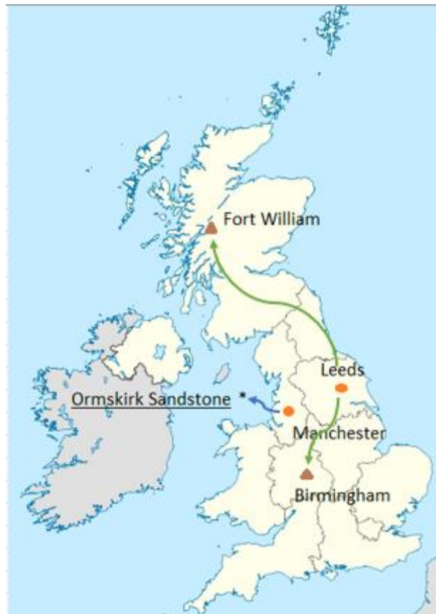
Figure 5 Topology of the optimized CCUS supply chain with Ormskirk Sandstone as storage site ( ● carbon dioxide source, * carbon dioxide storage, ▲ calcium carbonate production site, → to storage site, → to utilization site)
