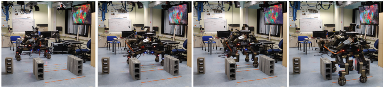
Fig. 12: Sequence of the CENTAURO robot narrowing into a passage, after starting from an expanded configuration.
