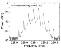
Fig. 7 Optical spectrum of the gain switched DML without OIL. The DML was biased at 52 mA.
