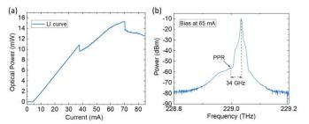
Fig.3 (a) Light-current (LI) curve of the cavity-enhanced laser; (b) Optical spectrum when biasing at 65 mA (resolution of 0.02 nm).
