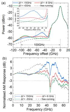
Fig. 5 (a) Optical spectra of the slave laser output with different OIL detuning frequencies; (b) Frequency responses (normalized at 0.4 GHz) at different OIL-DML detuning frequencies. The solitary results at 65 mA are plotted as the black dashed in as reference. The dip at 44 GHz is caused by a parasitic RF resonance of the chip-on-carrier
