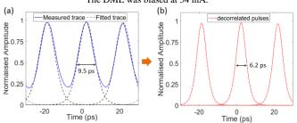
Fig. 10 Gain switching using the cavity-enhanced laser with OIL. (a) Measured autocorrelator results (blue curve) and the fitted pulse train (dashed curves) after removing the overlaps; (b) decorrelated pulses assuming Sech² pulse shape.
