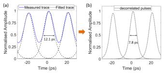
Fig. 8 Gain switching using the cavity-enhanced laser without OIL. (a) Measured autocorrelator results (blue curve) and the fitted pulse train (dashed curves) after removing the overlaps; (b) decorrelated pulses assuming Sech<sup>2</sup> pulse shape.
