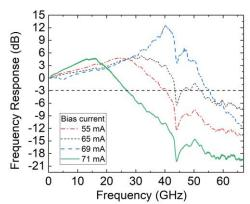
Fig. 4 Frequency responses of the cavity-enhanced laser at different bias current. Red Dash dot line: 55 mA; short dashed line: 65 mA; dashed line: 69 mA; Green solid line: 71 mA. The responses at low frequency (0.4 GHz) are normalized to 0 dB to compare the small-signal BW. The dip at 44 GHz is caused by a parasitic RF resonance of the chip-on-carrier.
