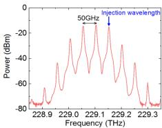
Fig. 9 Optical spectra of the gain-switched DML with OIL at 299.15 THz. The DML was biased at  $54\ mA$ .
