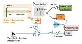
Fig.2 Experimental setup. Inset shows the laser structure. OSA: Optical spectrum analyzer; Amp.: RF amplifier; LCA: Lightwave Component Analyzer; PDFA: Praseodymium-Doped Fiber Amplifier; HR: high reflection; PC: polarization controller; DFB: distributed feedback.
