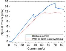
Fig. 6 Light-current measurement (LI curve) of the solitary laser under DC current drive (blue solid line) and 50-GHz gain switching (red dashed line).
