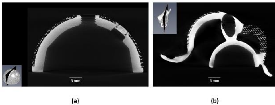
Figure A.1 – Micro-CT slice images of (a) off-the-shelf and (b) custom acetabular implants; the insert shows the location of the slice (scanning parameters: 180 kV – 80 \mu\text{A} )
