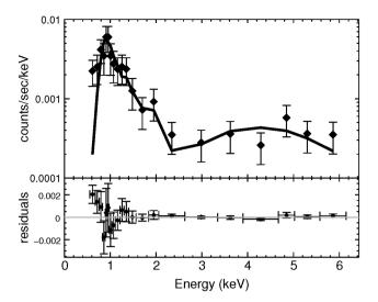
**Figure 3.** The background-subtracted X-ray spectrum obtained with Chandra on 2016 March 8–9, displayed with grouping to bins of at least 10 counts and fit with the 2-component soft+hard fit described in the text and Table 3. The fit itself was performed on the spectrum grouped to bins of at least 20 counts. The vertical axis is logarithmic for the spectrum and linear for the residuals.
