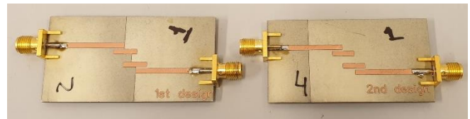
Fig. 5. The Photograph of the fabricated filters.
