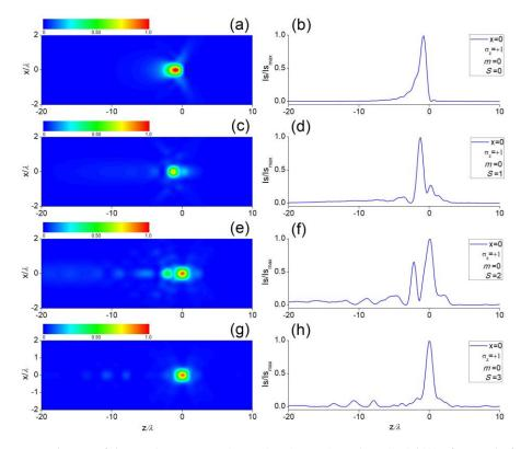
**Figure 10.** Evolution of the total intensity Is/Is<sub>max</sub> (2D (**a**,**c**,**e**,**g**), and 1D (**b**,**d**,**f**,**h**)) of strongly focused RHC ( $\sigma_z = +1$ ) polarized optical vortex  $LG_0^m$  (m = 0) regulated by a FCL of stage S = 0, 1, 2, and 3, respectively.
