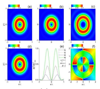
**Figure 4.** Calculated 2D distributions of  $|E|^2/|E|^2_{max}$  for a strongly focused RHC polarized ( $\sigma_z = +1$ ) optical vortex with charge m = +1, regulated by a FCL of S = 3: (**a**) *x*-polarized component, (**b**) *y*-polarized component, (**c**) *z*-polarized component, (**d**) total field, (**e**) line scan of focus, and (**f**) the helical phase structure of the longitudinal component of the focal electric field.
