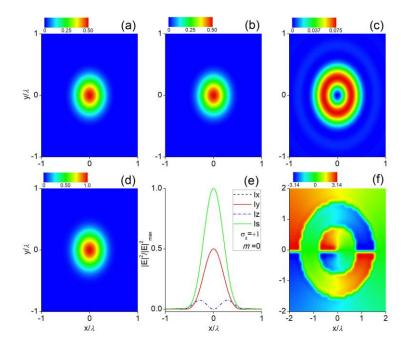
**Figure 2.** Calculated 2-D distributions  $|E|^2/|E|^2_{max}$  of a strongly focused RHC polarized ( $\sigma_z = +1$ ) optical vortex with charge m = 0, i.e., Gaussian beam, without a FCL: (**a**) *x*-polarized component, (**b**) *y*-polarized component, (**c**) *z*-polarized component, (**d**) total field, (**e**) line scan of focus, and (**f**) the helical phase structure of the *z*-polarized component of the focal electric field.
