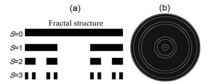
**Figure 1.** (a) Schematic of a 1-D fractal structure of a FCL following the triadic CS, starting from the stage S = 0 to S = 3; (b) schematic of 2-D fractal structure of a FCL (S = 3) following the triadic CS.
