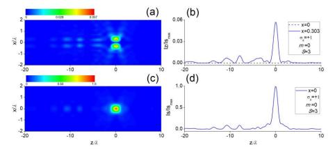
**Figure 7.** Evolution of the z-polarized component intensity  $Iz/Is_{max}$  (**a**,**b**) and total intensity  $Is/Is_{max}$  (**c**,**d**) (2D (**a**,**c**), and 1D **b**,**d**) of strongly focused RHC polarized ( $\sigma_z = +1$ ) optical vortex  $LG_0^m$  (m = 0), i.e., Gaussian beam, regulated by a FCL of stage S = 3.
