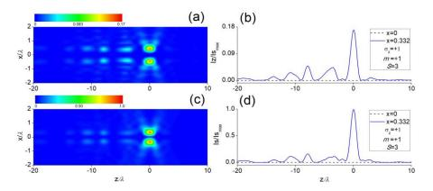
**Figure 8.** Evolution of the *z*-polarized component intensity  $Iz/Is_{max}$  (**a**,**b**) and total intensity  $Is/Is_{max}$  (**c**,**d**) (2D (**a**,**c**), and 1D (**b**,**d**)) of strongly focused RHC polarized ( $\sigma_z = +1$ ) optical vortex  $LG_0^m$  (m = +1) and  $\sigma_z = +1$  regulated by a FCL of stage S = 3.
