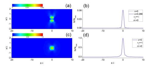
**Figure 6.** Evolution of the z-polarized component intensity  $Iz/Is_{max}$  (**a**,**b**) and the total intensity  $Is/Is_{max}$  (**c**,**d**) (2D (**a**,c), and 1D (**b**,**d**)) of strongly focused RHC polarized ( $\sigma_z = +1$ ) optical vortex  $LG_0^m$  (m = 0), i.e., Gaussian beam, without a FCL.
