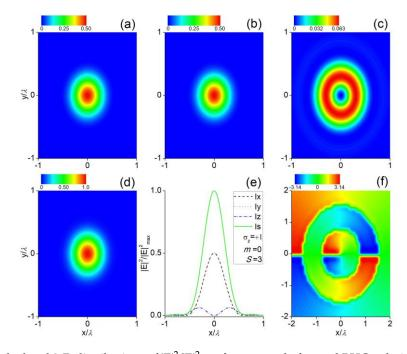
**Figure 3.** Calculated 2-D distributions of  $|\mathbf{E}|^2/|\mathbf{E}|^2_{\max}$  for a strongly focused RHC polarized ( $\sigma_z = +1$ ) optical vortex with charge m = 0, i.e., Gaussian beam, regulated by a FCL of S = 3: (a) *x*-polarized component, (b) *y*-polarized component, (c) *z*-polarized component, (d) total field, (e) line scan of focus, and (f) the helical phase structure of the longitudinal component of the focal electric field.
