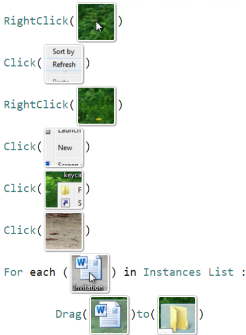
Figure 14. The system successfully use videos as input of the system, instead of generating the input log-file from the sniffer, to create a working script. Please note that the system failed to remove mouse pointer from the target patterns in the first and the seventh lines.
