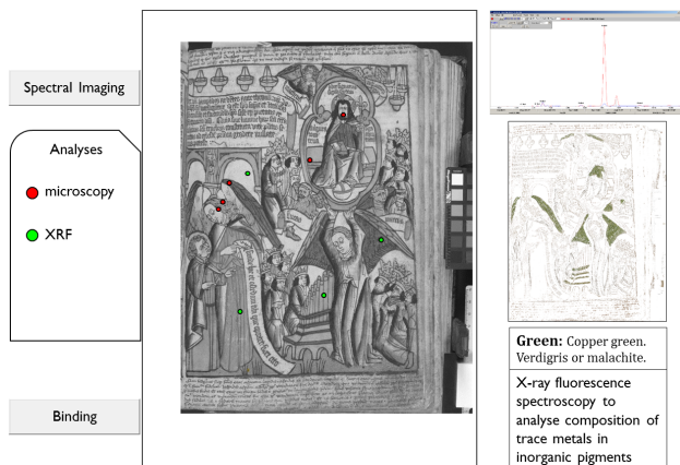
Figure 2. Creating spatially located X-Ray Fluorescence (XRF) data linked as annotation layers
