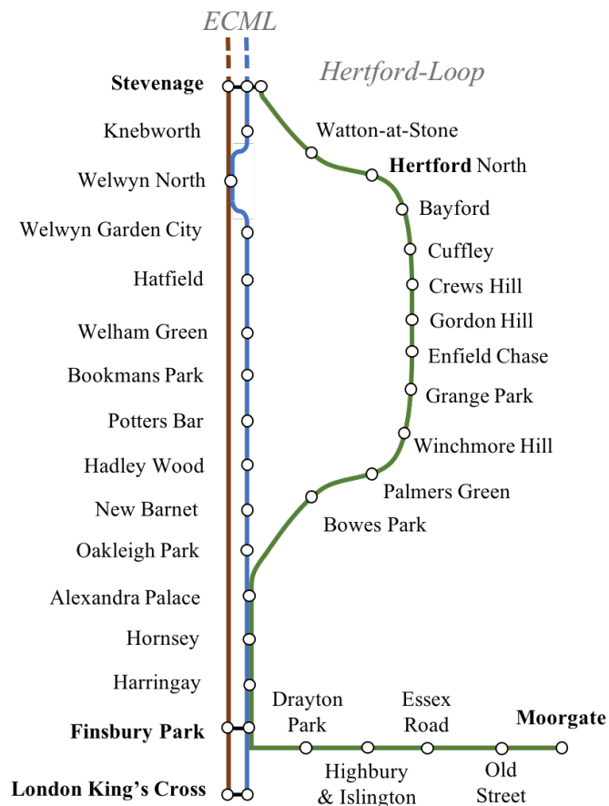
Figure 5.1: Schematic of the southbound, southern section of the East Coast Main Line. Different colours of track present particular services, with varying train mechanical capabilities, stopping patterns and train operators.
