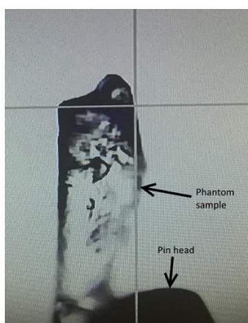
Figure 24. Light microscopy image of sample of phantom mounted on pin head. The phantom is assessed on its geometry to ensure it is neither too big nor too small to be imaged.
