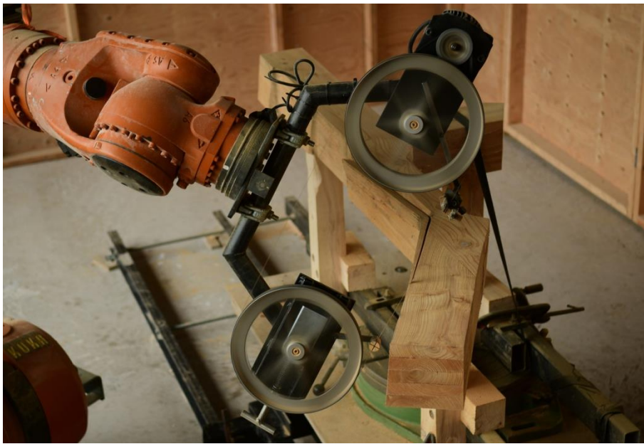
Fig. 3. Weapon of choice - bandsaw end effector used during ‘Bandsaw Manoeuvres’
