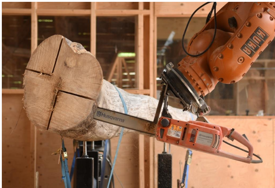
Fig. 4. Weapon of choice - chainsaw end effector used during 'Chainsaw Choreographies'
