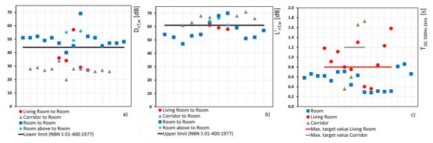
Figure 4 - Building acoustic performance measured in the five nursing homes, ante operam:  $D_{nT,w}(a)$ ,  $L'_{nT,w}(b)$ , and  $T_{500Hz-2kHz}(c)$ .
