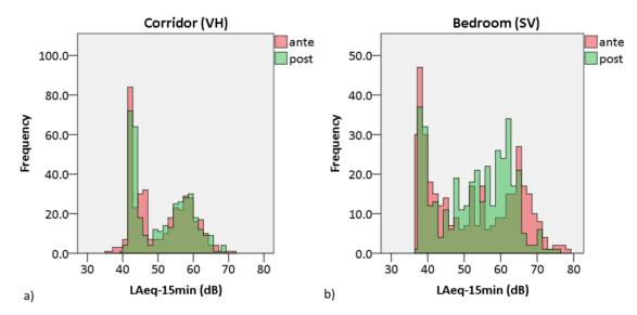
Figure 7 – Noise levels distributions for the ante and post operam conditions in a corridor in VH (a) and a bedroom in SV (b)
