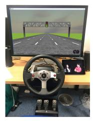
Figure 1: Driving simulator setup with steering wheel, pedals, monitor, and iPad for secondary task.
