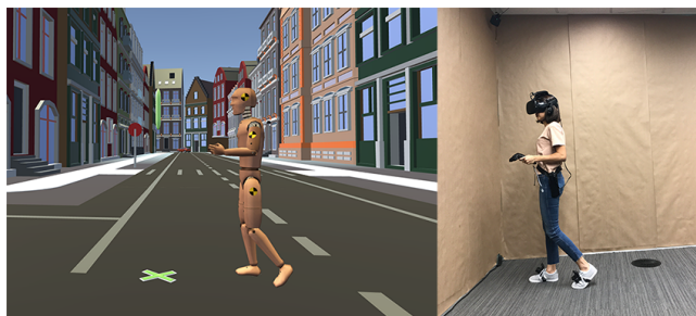
Figure 1: Participant walking towards a target before the distance estimation task. Left) The avatar and the green target in the virtual city. Right) Participant holding the controllers while wearing the battery pack, wireless HMD, and foot trackers.
