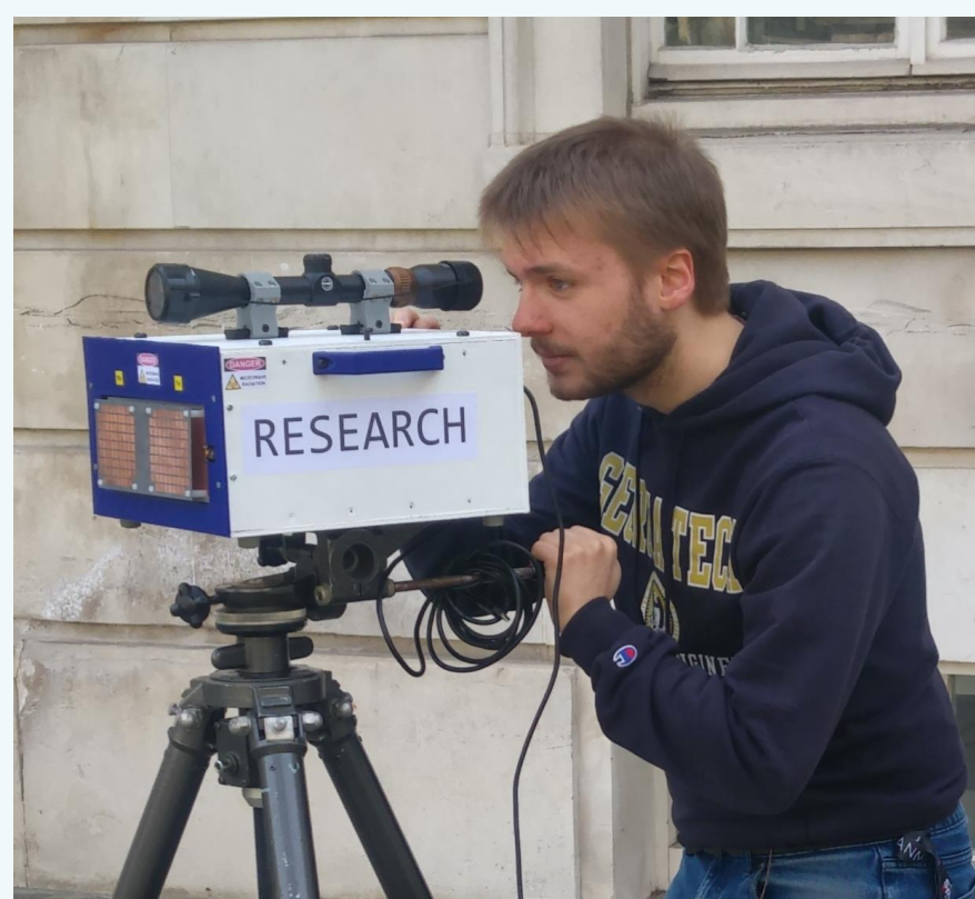
Packaged FMCW radar unit during field trials
