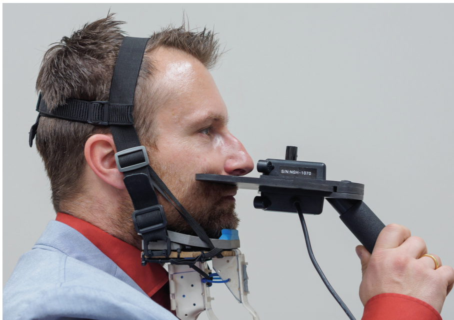
Figure 1 - An example of the experimental setup used to determine the independent effects of nasalization on the vowel space, including a hand-held Glottal Enterprises nasalance device and an ultrasound probe holder headset (Derrick et al., 2015). Reproduced from Carignan (2018)
