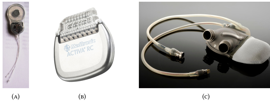
FIGURE 1.3: Modern IMDs, (A): A Nucleus cochlear implant, (B): An Activa RC neurostimulator from Medtronic, and (C): A prototype Heartsaver ventricular assist device (VAD). 3
