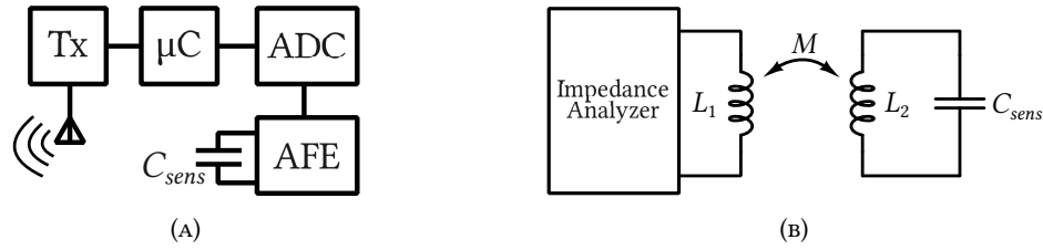
FIGURE 4.1: Typical sensor architectures. (A): a typical remote sensor chain with digital wireless transmitter. (B): an inductive link based remote interrogator, using an impedance analyzer.
