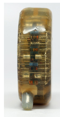
FIGURE 1.2: The Chardack-Greatbatch pacemaker, (A) front and (B) side view. Reproduced with permission. 2
