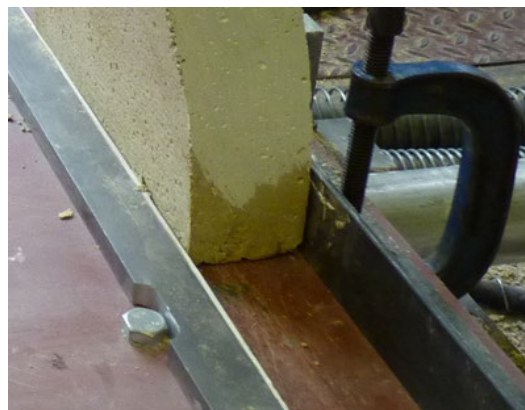
Fig. 4. Support conditions for arch samples on shaking table with rubber padded metal brackets on both intrados and extrados to prevent sliding, while a degree of rotation can be expected.
