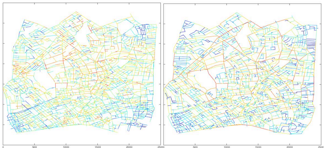
Fig 2: RWB for Barnsbury and surroundings. The left map uses a transition probability in proportion to the angular weight, the right uses angular weight ^4 . Colour values for RWB are logarithmically scaled.
