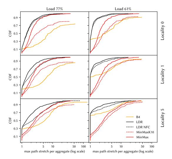
**Figure 7.9:** Maximum flow stretch under different load and locality values; LLPD > 0.5; no headroom; where the CDF fails to reach 1.0, this indicates that in the remaining scenarios the routing system could not find a placement that would fit all the traffic
