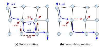
**Figure 3.4:** Greedy routing yields high delay on mesh-like networks; all links have a capacity of one unit and the two aggregates have a demand of one unit. The long-haul aggregate (shown in blue) has a second best path that is of slightly longer latency than its shortest path, while the second best path of the local aggregate (show in red) is significantly worse.
