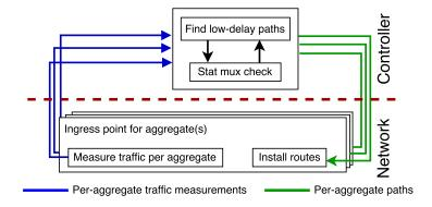
Figure 4.3: High-level operation: controller and ingress points.
