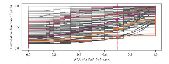
**Figure 3.6:** CDF curves of APA for all networks, given path stretch limit of 40%. Five random curves are highlighted. The vertical line at 0.7 indicates PoPs 70% of whose shortest-path links can be routed around without excessive delay.
