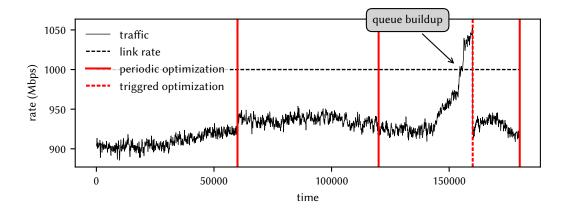
**Figure 7.23:** Traffic that crosses link rank 20 from Figure 7.22; time is in milliseconds; traffic is binned in 100 ms bins and each point is the mean of a bin. In this experiment LDR is given the exact mean traffic levels for the upcoming minute, but this knowledge of the future is of little use as the unexpected change happens mid-minute.
