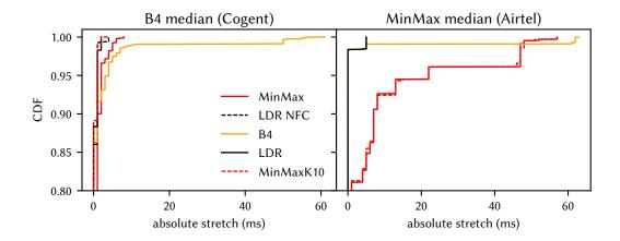
Figure 7.11: Absolute stretch in median topologies; only showing the top 20% of each distribution.
