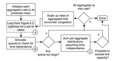
Figure 6.1: Picking rates to cope with short-term variability. Initially each aggregate's level is set to that of its predicted mean (see Section 6.2.3), the optimizer is then run (A) and the solution is checked for temporally correlated events (B) and whether multiplexed traffic is likely to overflow any queue in the network (C). If either of those is true the levels of aggregates that are likely to experience congestion are moved closer to their maximum and the process repeats.
