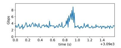
Figure 3.16: A short-term spike in traffic level; from 2016 CAIDA packet trace of uncongested U.S. Tier-1 ISP link.
