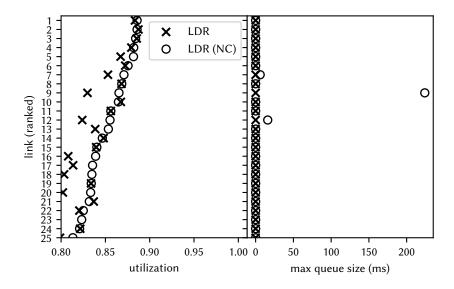
**Figure 7.28:** Mean link utilization (left) and max queue size (right) for the first ten minutes; 10% headroom target for the mean level estimation algorithm; limited optimization enabled. Links are ranked based on the utilization of LDR (NC).
