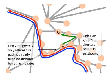
**Figure 3.10:** Inadvertent congestion on GTS using B4. The greedy nature of B4's path allocation causes both directions of the first link on the  $V \rightarrow G$  path to quickly become saturated, at which point there are no alternative paths for the  $V \rightarrow G$  traffic.
