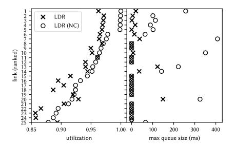
**Figure 7.22:** Perfect next-minute mean level prediction; convolution algorithm uses previous minute's traffic to assess short-term variability. Mean link utilization (left) and max queue size (right) for the first three minutes. Links are ranked based on the utilization of LDR (NC).
