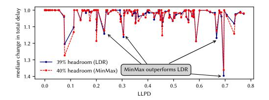
Figure 7.15: Sub-optimality with LDR. Plot shows median latency stretch at 39% and 40% headroom. The two curves are for LDR and MinMax, which is the optimal multi-commodity flow solution that minimizes link utilization.
