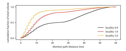
Figure 7.6: Cumulative fraction of total volume in Cogent's topology that travels a given shortest-path distance.
