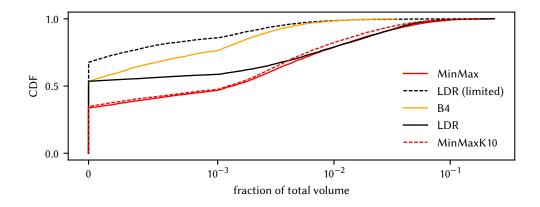
**Figure 7.16:** CDF of the fraction of total network volume that changed paths. Each point is a separate traffic matrix, the load of whose aggregates is randomly uniformly distributed +/- 5%.
