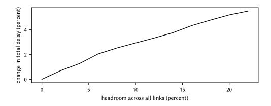
Figure 7.25: Increase in delay due to adding a fixed amount of headroom to all links.
