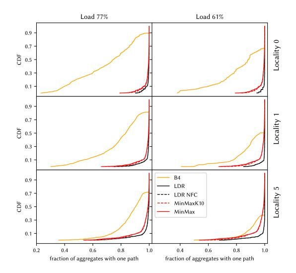
Figure 7.13: Fraction of aggregates that have only one path under different load and locality values; LLPD > 0.5; no headroom
