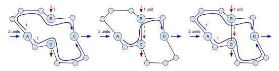
(a) Initial scenario.(b) Minimal propagation delay; (c) Longer propagation delay; no congestion at A.
