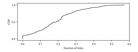
Figure 3.1: CDF of the fraction of links that, when removed from each topology, converts it into a spanning tree; 237 real-world topologies from the Topology Zoo [50] dataset.
