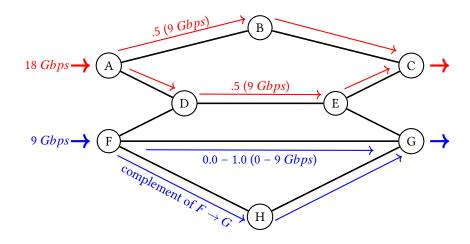
**Figure 2.5:** All links are 10 Gbps; MinMax can fail to minimize utilization in links with utilization below the utilization of the link with minimum maximal utilization; the MinMax utilization is 0.9, the split of bottom aggregate is undefined.
