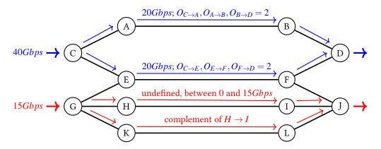
**Figure 5.1:** All links are 10 Gbps;  $O_{max} = 2$ , attained at the top links. If the optimizer uses the objective in 5.1 the bottom aggregate's traffic may end up congesting one of the bottom paths even though there is capacity for it to fit.
