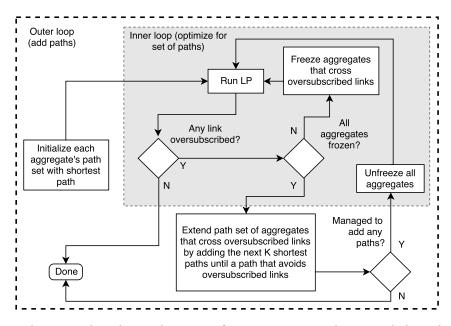
**Figure 5.3:** Obtaining paths and per-path aggregate fractions, assuming each aggregate's demand is known. This is a two-stage process: the inner loop uses Equation 5.3 to minimize both delay and oversubscription for a given set of paths (Section 5.2) and the outer loop adds new paths (Section 5.3).
