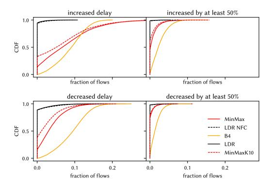
Figure 8.3: Fraction of flows whose delay increases/decreases when an existing link is upgraded in Hurricane Electric's network
