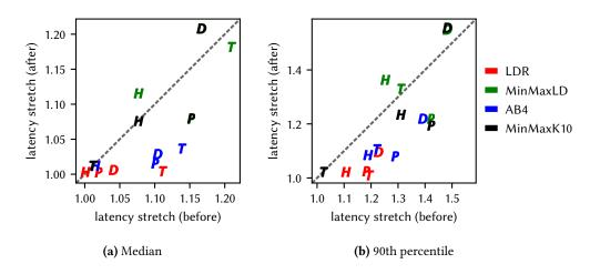
**Figure 8.2:** Latency benefits of network growth; graph shows median and 90th percentile of path stretch before and after growing networks to increase their LLPD; each letter is a different topology: Packetexchange (P), Deutsche Telekom (D), Hurricane Electric (H) and Tinet (T).
