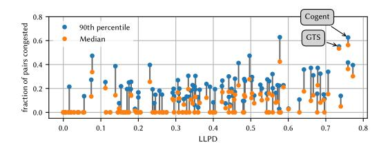
**Figure 3.8:** Networks with high LLPD tend to concentrate traffic when using SP routing. The *x*-axis shows the topologies sorted according to their LLPD, and the *y*-axis reports the fraction of source-destination pairs that experience congestion.
