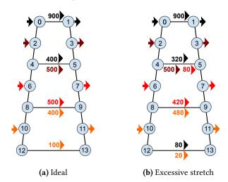
**Figure 4.2:** The solution to the left is the same as the ideal one in Figure 4.1d. The solution to the right has the same total propagation delay as the one on the left, but is less desirable due to excessive stretch.
