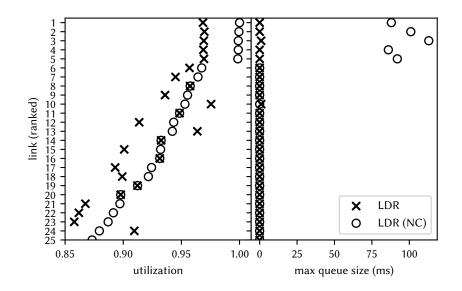
**Figure 7.21:** Perfect next-minute mean level prediction; convolution algorithm has access to current traffic counters. Mean link utilization (left) and maximum queue size (right) for the first minute. Links are ranked based on the utilization of LDR (NC).
