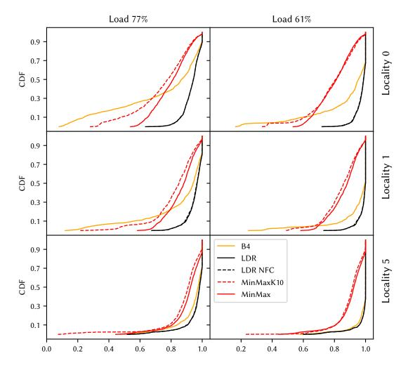
Figure 7.10: Fraction of flows that are routed on the shortest path under different load and locality values; LLPD > 0.5; no headroom
