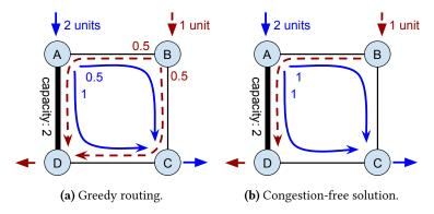
**Figure 3.3:** Greedy routing gets stuck in local minimum, fails to avoid congestion; all links have the same delay and the same unit capacity, except for  $A \rightarrow D$ , whose capacity is 2 units.
