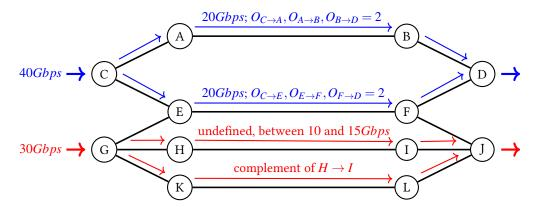
**Figure 5.2:** Same scenario as in Figure 5.1, but the bottom aggregate's demand is 30*Gbps* and not satisfiable by the two bottom paths. This creates two regions of different oversubscription in the network. A single application of Equation 5.3 will minimize oversubscription in the top part of the network, but not in the bottom one.
