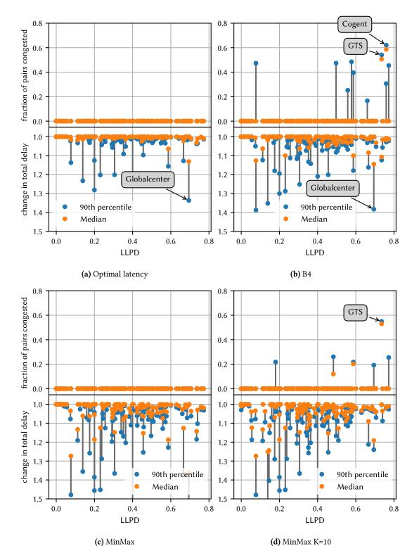
**Figure 3.9:** Effects of active routing on congestion and delay. The top part of each graph shows the fraction of all non-zero demands in the traffic matrix that end up crossing at least one congested path, the bottom part shows latency stretch. For each *x* value (different topology) we plot the median and 90th percentile from runs across a range of traffic matrices. The gray line indicates the span of the distribution.
