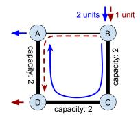
**Figure 3.5:** Congestion-free solution that is unattainable by SP routing regardless of assignment of weights; thick lines have a capacity of 2 units.
