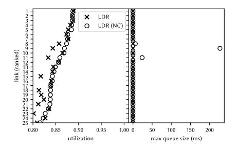
Figure 7.26: Mean link utilization (left) and max queue size (right) for the first ten minutes; 10% headroom target for the mean level estimation algorithm. Links are ranked based on the utilization of LDR (NC).
