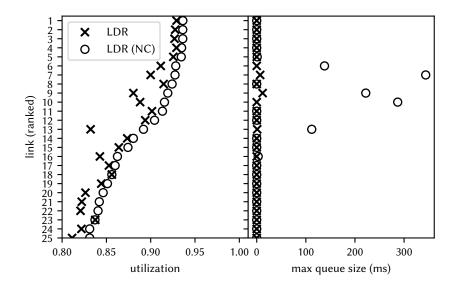
Figure 7.27: Mean link utilization (left) and max queue size (right) for the first ten minutes; 5% headroom target for the mean level estimation algorithm. Links are ranked based on the utilization of LDR (NC).
