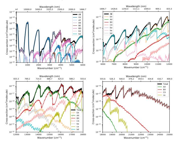
Figure 7. Decomposition of the total cross-section of TiO using TOTO below 25000 cm<sup>-1</sup> into the main bands for an assumed temperature of 2000 K. Individual lines have been broadened with a Gaussian profile with a half width at half-maximum (HWHM) of 2 cm<sup>-1</sup>, T = 2000 K. Note that different *y*-axis scales have been used for each sub-figure.
