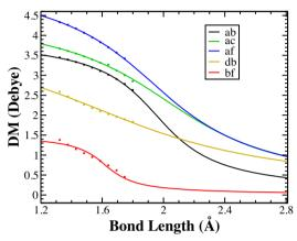
Figure 6. Ab initio off-diagonal dipole moment for singlets in crosses from Langhoff (1997), and the fitted curves (this work) in continuous curves.
