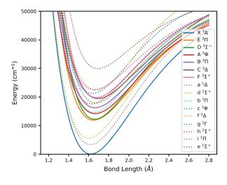
Figure 1. Fitted PECs for <sup>48</sup>Ti<sup>16</sup>O.
