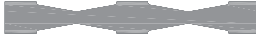
Fig. 17. Two geometries of WHPs giving the same strength but with different yield displacements.
