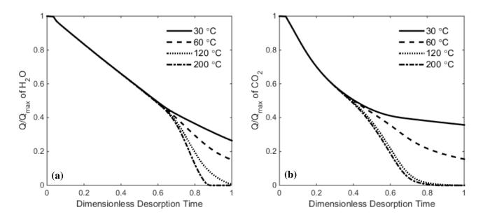
Fig. 11 Variation of dimensionless total adsorbed amount in the bed for H<sub>2</sub>O and CO<sub>2</sub> with dimensionless
