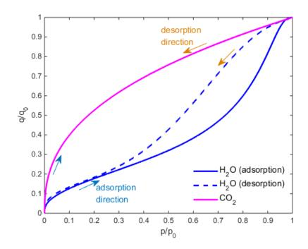
Fig. 9 Dimensionless adsorption/desorption isotherm for  $H_2O$  and  $CO_2$  at 30  $\,^\circ\!\mathrm{C}$
