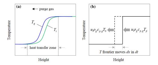
**Fig. 12** Energy balance analysis on an elementary volume of the bed during purge step (**Fig. a**: normal temperature profile along the bed height; **Fig. b**: idealized temperature profile along the bed height neglecting
