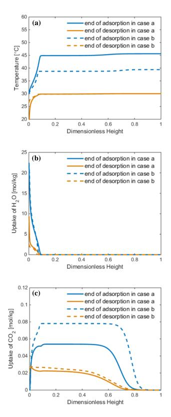
Fig. 7 Distribution of temperature and uptakes of H<sub>2</sub>O and CO<sub>2</sub> along the bed height at the ends of feed step
