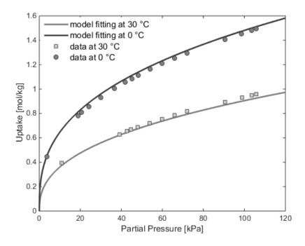
Fig. 3 Fitting of CO<sub>2</sub> adsorption isotherm data on alumina F200.
