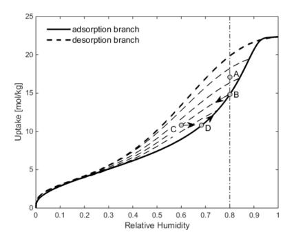
Fig. 4 Different branches of the  $H_2O$  desorption isotherm at 30  $^\circ\!{\rm C}.$
