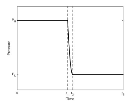
**Fig. 1** Pressure change with time in the studied cycle  $(0 \sim t_1 \text{ is feed step}, t_1 \sim t_2 \text{ is blowdown step}, t_2 \sim t_3 \text{ is}$
