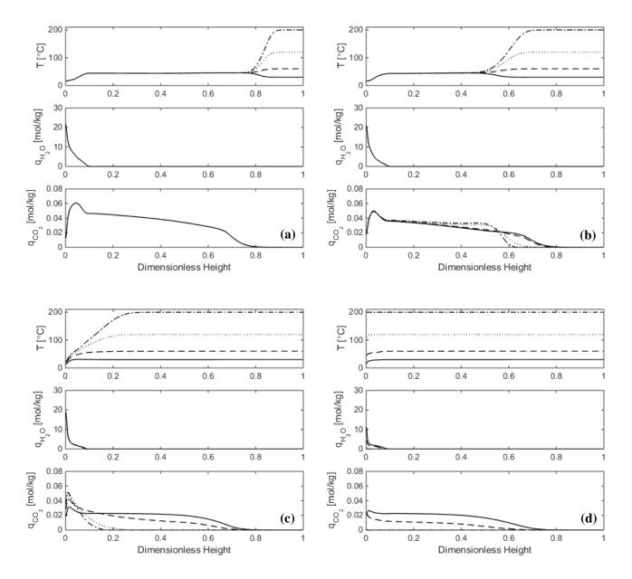
**Fig. 10** Distribution of temperature and uptakes of H<sub>2</sub>O and CO<sub>2</sub> along the bed height at 1/6, 1/3, 2/3 and 1/1 of desorption time in case a (solid lines, 30 °C; dashed lines, 60 °C; dotted lines, 120 °C; dash-dotted lines,
