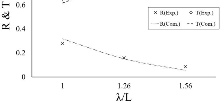
Fig 4 Computational and experimental R & T, as a function of wavelength divided by ice length.
