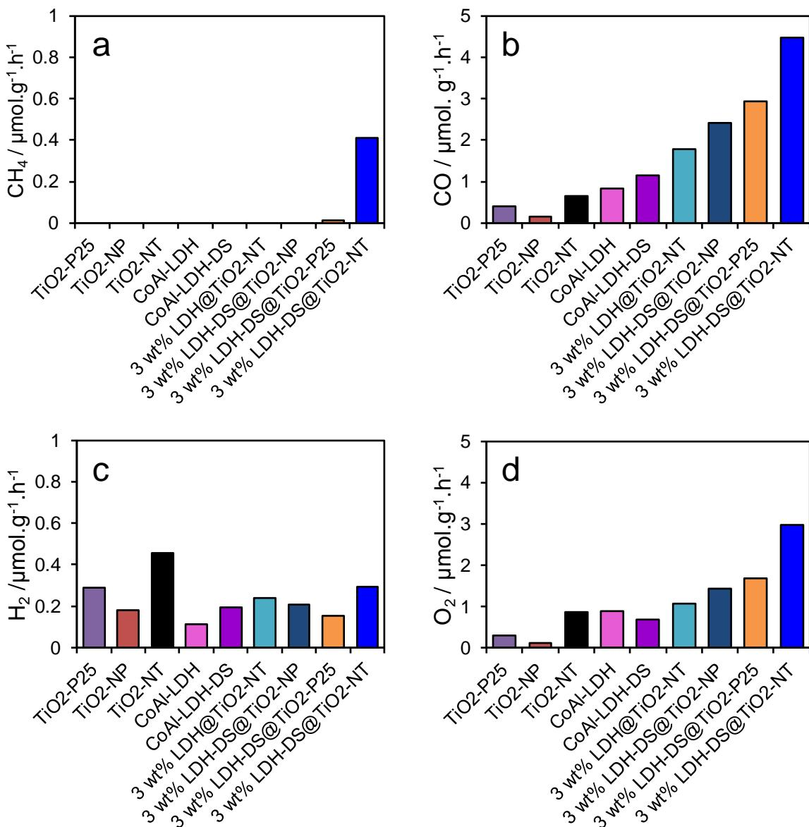
**Figure 4.** (a)  $\text{CH}_4$ , (b)  $\text{CO}$ , (c)  $\text{H}_2$  and (d)  $\text{O}_2$  mass-normalized productivity averaged over the first 4 h of aqueous phase  $\text{CO}_2$  photoreduction over 3 wt% LDH-DS@ $\text{TiO}_2$  nanocomposites, and CoAl-LDH and  $\text{TiO}_2$  references under UV-Vis irradiation by a 300 W Xe lamp.
