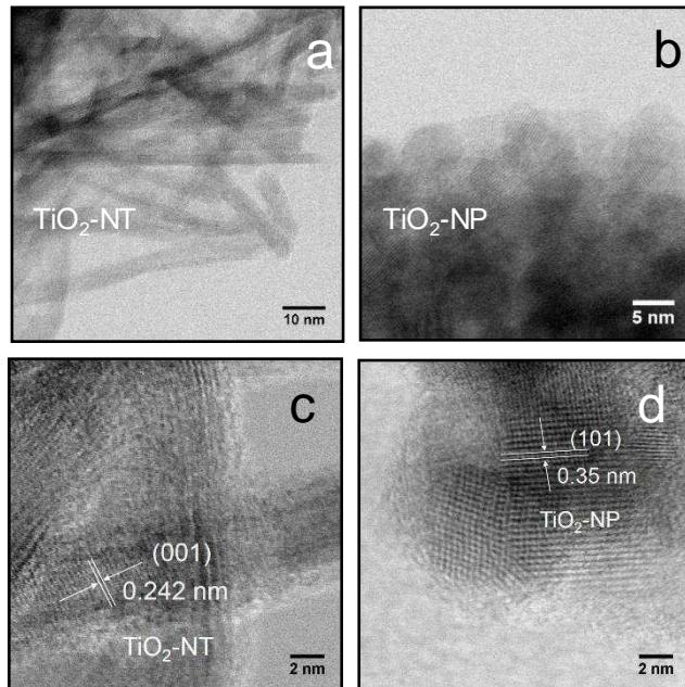
**Figure 2.** Low and high resolution TEM images of (a,c) TiO<sub>2</sub>-NT, and (b,d) TiO<sub>2</sub>-NT.
