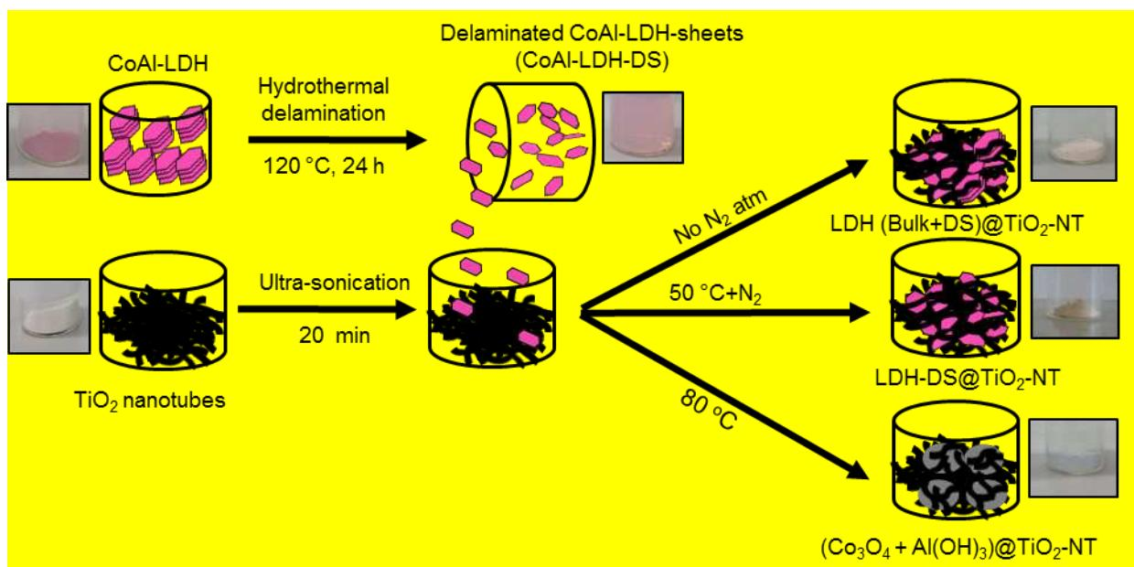
**Scheme 1.** Schematic of CoAl-LDH@TiO<sub>2</sub> nanocomposite synthesis.
