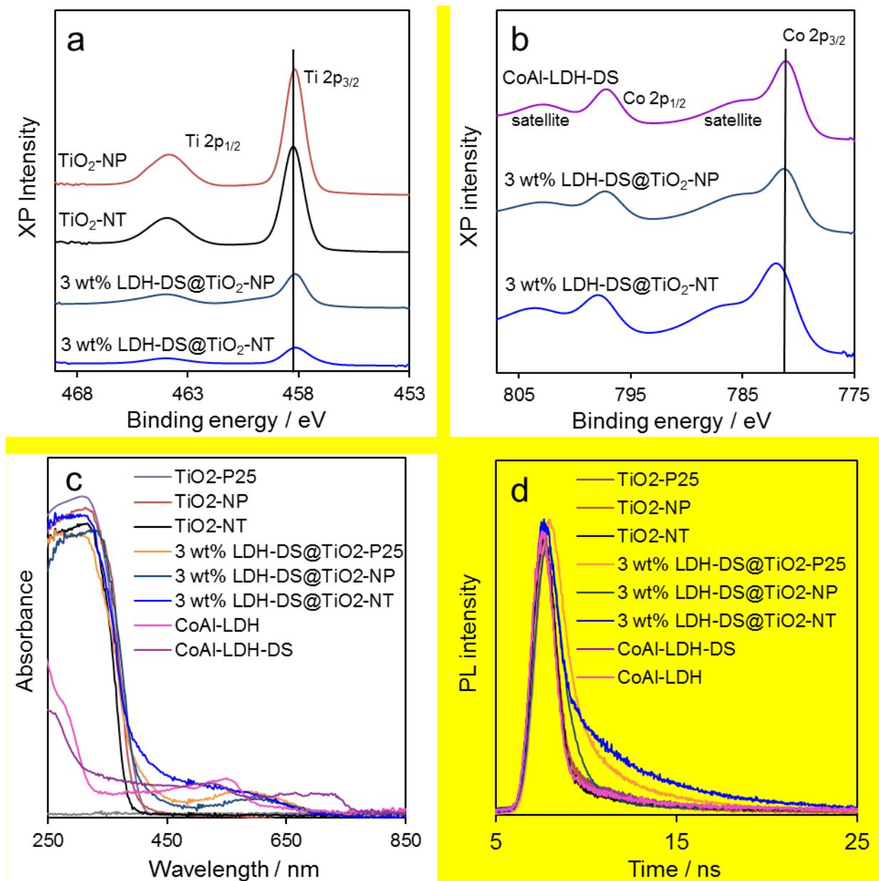
**Figure 3.** (a) Ti 2p and (b) Co 2p XP spectra, (c) DRUVS, and (d) time-resolved PL spectra at 380 nm excitation wavelength of 3 wt% LDH-DS@TiO<sub>2</sub> nanocomposites alongside CoAl-LDH and TiO<sub>2</sub> references.
