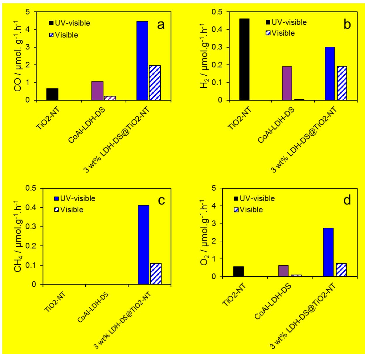
**Figure 5.** Comparison of (a) CH<sub>4</sub>, (b) CO, (c) H<sub>2</sub> and (d) O<sub>2</sub> mass-normalized productivity averaged over the first 4 h of aqueous phase CO<sub>2</sub> photoreduction over 3 wt% LDH-DS@TiO<sub>2</sub>-NT nanocomposite, and CoAl-LDH-DS and TiO<sub>2</sub>-NT references under UV-Vis versus visible only light irradiation.
