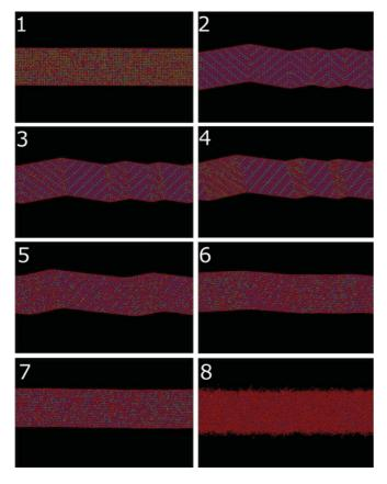
FIG. 4. (Color online) A visualization of the complete cool-load-reheat cycle performed on an ensemble of 80 000 atoms. A movie of this sequence is available in online supplementary materials.<sup>45</sup>
