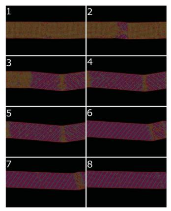
FIG. 5. (Color online) Images of the system being at T = 75 after applying total shears of  $\Sigma \epsilon$  0.001, 0.003, 0.009, 0.022, 0.035, 0.051, 0.072, and 0.08, respectively. Snapshots are noisy at these temperatures, so each image is based on samples where the shearing was stopped for 500 time steps to allow equilibration, and then average positions were taken over 100 time steps. A movie of this sequence is available in online supplementary materials.<sup>45</sup>
