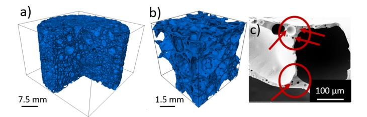
**Fig. 1.** 3D micrographic reconstructions of the pore structure of glass foam prepared without K<sub>3</sub>PO<sub>4</sub> in a) full-size, b) subvolume, and c) SEM secondary electron image of struts (marked by circles), pore walls, and small pores inside struts (marked by arrows).
