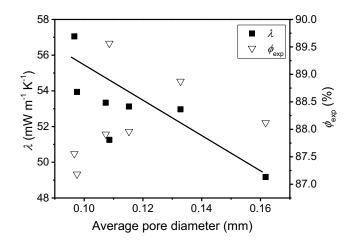
Fig. 4. Change in thermal conductivity ( $\lambda$ ) and porosity ( $\phi_{exp}$ ) with increasing average pore diameter based on D<sub>eq</sub>. Errors of  $\lambda$  and  $\phi_{exp}$  are 0.1 mW m<sup>-1</sup> K<sup>-1</sup> and 0.1 point, respectively. The error of pore diameter is ±0.1 mm. The line is intended as visual guideline.
