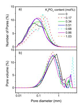
**Fig. 2.** Distribution of pore size (equivalent sphere diameter) of glass foams with different K<sub>3</sub>PO<sub>4</sub> content (XMT data). a) Number of pores with bimodal distributions shown as dashed lines and b) pore volume. The pore diameter is in log space.
