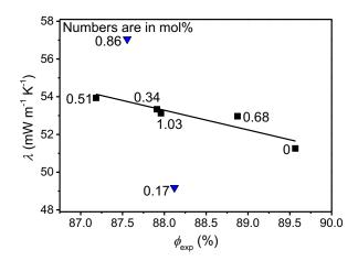
Fig. 3. Change in thermal conductivity ( $\lambda$ ) with the porosity ( $\phi_{exp}$ ). The labels refer to the K<sub>3</sub>PO<sub>4</sub> content. Outliers are marked with triangles. The errors are smaller than the symbols. The line is a visual guideline.
