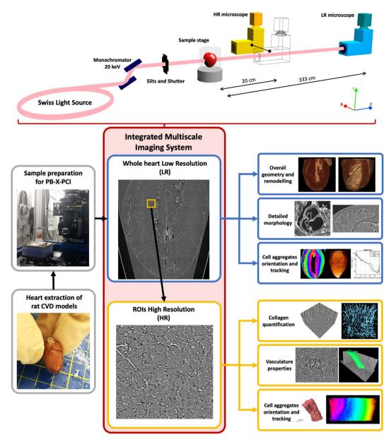
**Figure 1.** Multiscale imaging and analysis of cardiac tissue. Diagram describing the processing pipeline and imaging setup of the methodology used for comprehensive cardiac tissue analysis.
