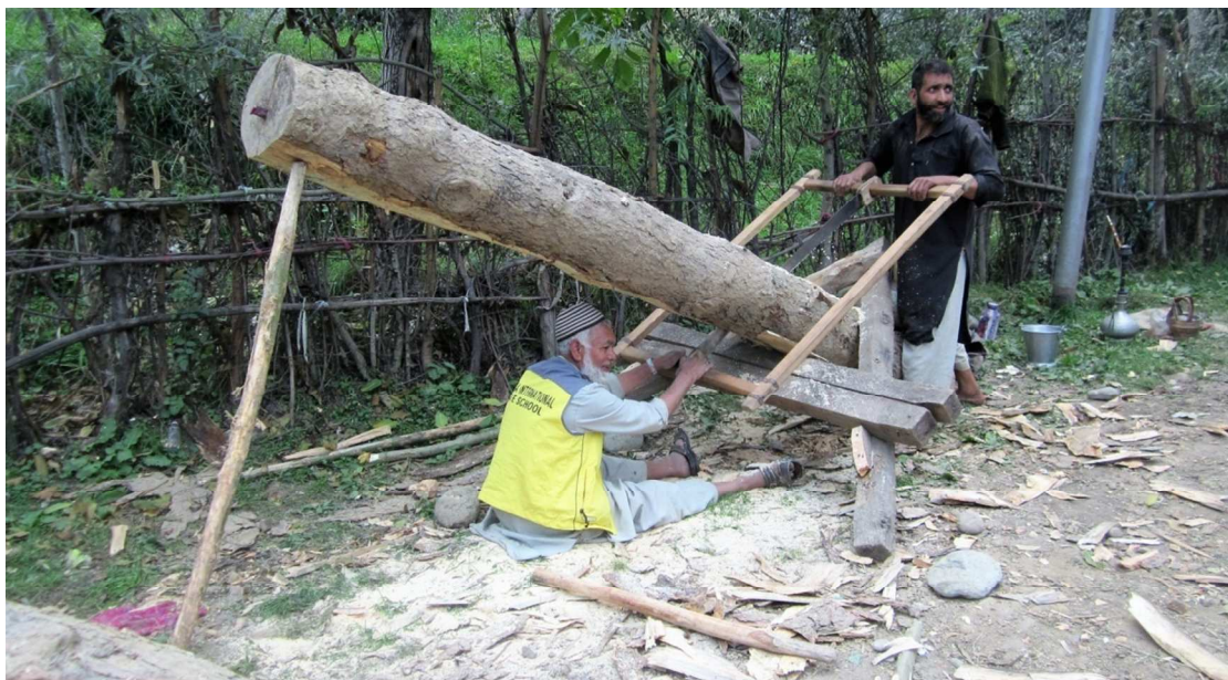
Fig. 4. Men at work together using a cross-cut saw. Use of this locally available technology is still common in the villages of Kashmir Valley.
