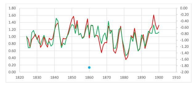
Figure 5. Indexed average ring width values for Control (green) and Symptomatic (red) trees at SC, the start of a phase of cool summers in 1860 is indicated, in comparison to the long-term average summer temperature (Central England Temperature, Parker et al 1992).
