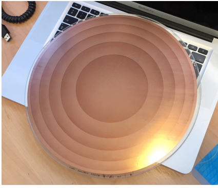
Figure 2. The completed 300mm metal mesh Fresnel lens.
