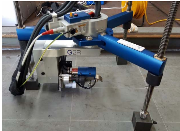
Figure 12. The set-up of the XRD (X-Ray Diffraction technique) technique to measure the welding-induced residual stresses.
