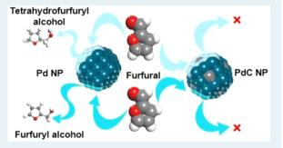
furfuryl alcohol. We demonstrate, through combined experimental and computational studies, that Pd nanoparticle planes are more prone to deactivation through the formation of Pd carbide, resulting in the reduced efficacy of furfural binding. This approach to nanoparticle optimization is an important strategy for producing long-lasting, high-performance catalysts for emerging sustainable technologies.
