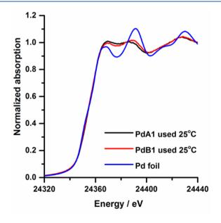
Figure 6. Normalized XANES spectra of PdA1 and PdB1 after catalysis and a Pd<sup>0</sup> reference.
