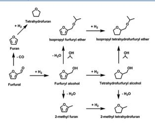
**Figure 1.** Schematic representation of reaction pathways during furfural hydrogenation.
