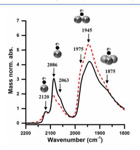
Figure 3. FTIR spectra from CO adsorption studies on PdB1 (solid black line) and PdA1 (red dashed line).
