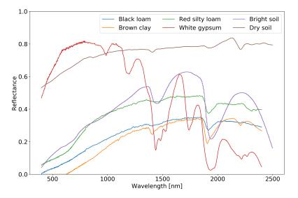
**Figure 2.** 6 soil spectra chosen to reflect varying absorption features taken from Baldridge et al. [24] and Price [23].
