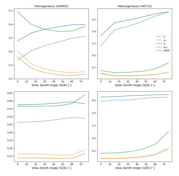
**Figure 5.** Dependence of *a*, *p* and DASF with Solar Zenith Angle (SZA) (**top panels**) and View Zenith Angle (VZA) (**bottom panels**) for homogeneous (**left panels**) and heterogeneous (**right panels**) canopies.
