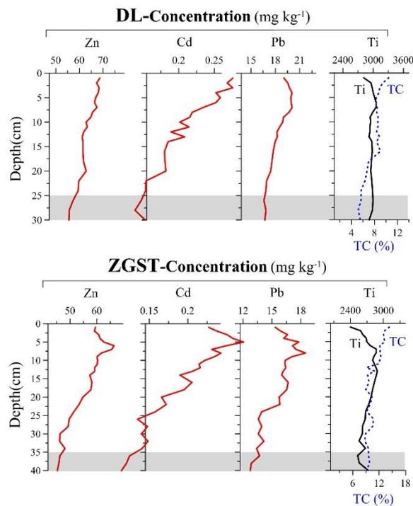
**Fig. 2** Heavy metal concentrations, Ti, and TC in sediment cores from lakes of DL and ZGST. For comparison, their X axes are set at the same range of  $3/4 * \text{Average}[C_i] \leq X \leq 5/4 * \text{Average}[C_i]$ .
