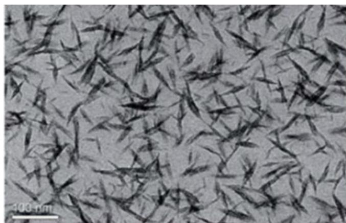
Figure 7. A TEM image of \text{TiO}_2 nanoparticles prepared via SPP method.
