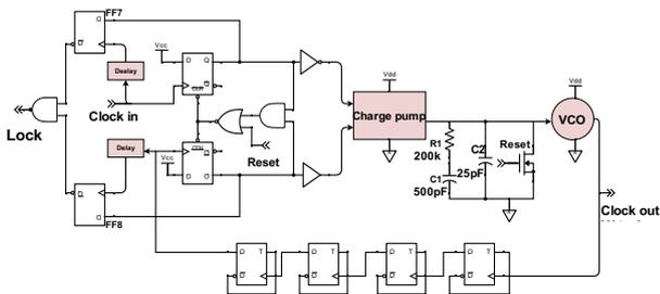
Fig. 4: Phased-locked loop and lock generation circuit.
