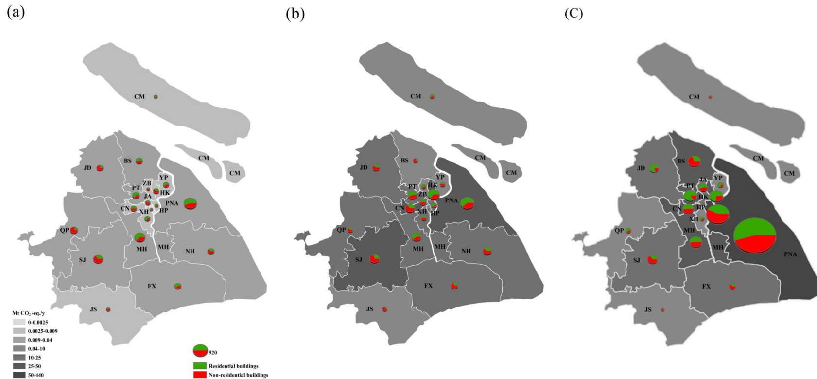
Fig.9. Spatial distribution of building area and embodied GHG emissions in Shanghai in 2003(a), 2008(b) and 2016(c)
