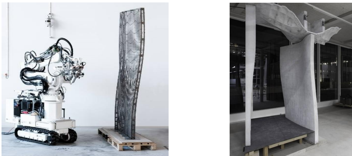
255 256 Figure 3. Prototype of double-curved wall built with the Mesh Mould process. IF and MMW (left) and finished wall (right) 257 (source: NCCR Digital Fabrication, 2017)
