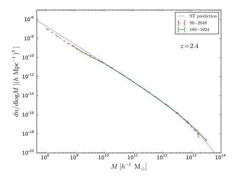
**Figure 1**: Halo mass functions of the 80-2048 simulation (red dashed line) and of the 160-1024 simulation (green solid line) compared with the Sheth-Tormen prediction [24] (blue dotted line). The error bars are the uncertainties in each of the mass bins used for the computation assuming that the number of halos follows a Poissonian distribution.
