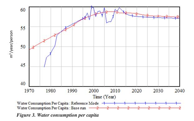
**Figure 3** exhibits how simulated water consumption per capita has increased since year 1970 until year 2010, and then it decreases reaching stabilization. This behaviour sufficiently replicates the reference mode.
