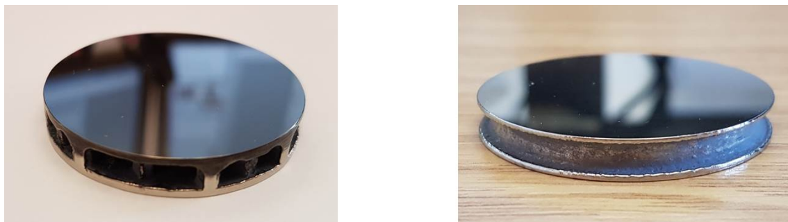
Figure 11. A comparison between the polished non-optimised ( left ) and optimised ( right ) mirror samples.
