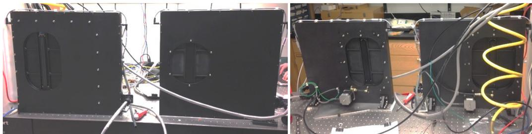
Figure 17: The shutter assemblies shown in the closed position with the exposure shutter on the left and the NIR shutter on the right. The views show the front (left) and reverse (right) sides of the shutters. The fiber illuminator LED is visible in the exposure shutter door front view. The motor and inflatable seal mechanism is visible in the reverse view.
